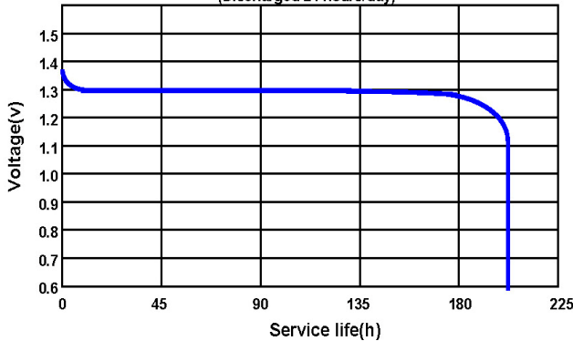
DISCHARGE CHARACTERISTICS AT 1500Ω 20°C 60% RH (Discharged 24 hours/day)
